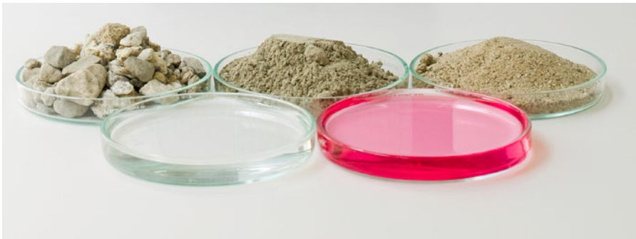
Fig. 4.2.2: Mix design ingredients of concrete: Coarse aggregates, water, cement, superplasticizer, sand (from left to right)
