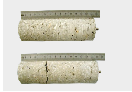
Fig. 8.4.1: Concrete deterioration due to sulfate attack shows a strong increase in length because of the spalling attack. First cracks have appeared in sample.
