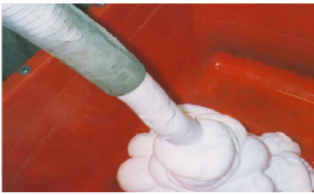
Fig. 8.15.2: Foam generated by a foam generator and Sika® Stabilizer Poro to produce cellular / foam concrete.
