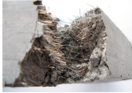
Fig. 8.9.1: High strength and above all ultra high performance concrete (UHPC) are usually fiber-reinforced. Depending on the requirements, synthetic and/or steel fibers are thereby employed in large quantity.
