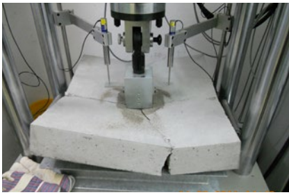
Fig. 8.11.3: Special testing for sprayed concrete: Energy absorption testing of fiber reinforced sprayed concrete to EN 14488-5.
