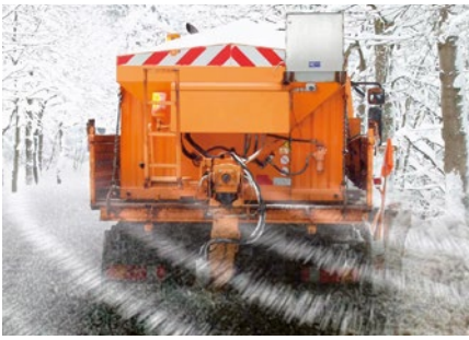
Fig. 8.3.3: Scattered de-icing agent considerably intensifies the reaction upon freezing of water and leads to substantially greater damage in areas of concrete close to the surface.
