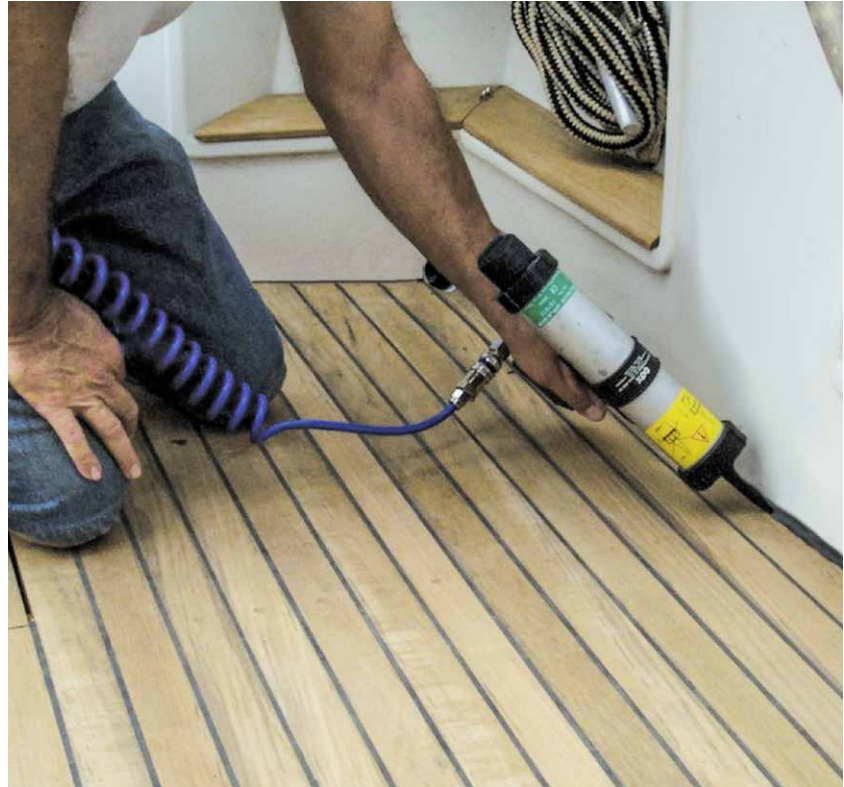
Fig. 25 Sealing the edges after renovation with Sikaflex®-295 UV
