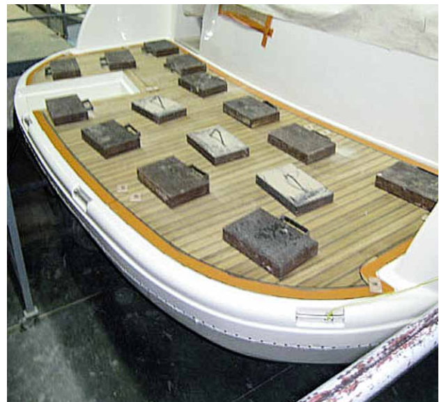
Fig. 27 Holding in place with weights
