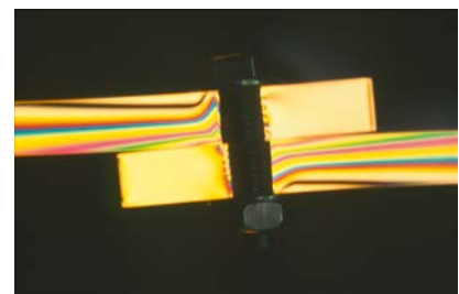
Fig. 4 Screwed sample. The force line indicate a direct transmission of the forces from one part of the sample through the screw to the other part of the sample
