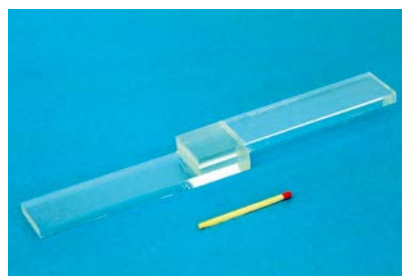
Fig. 3 Test sample. Lap shear test with PMMA substrate bonded with different adhesives. One sample has been screwed
